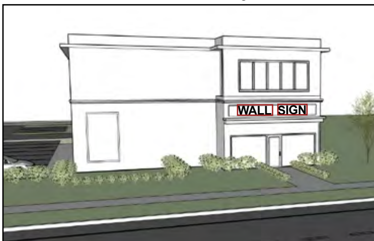
155.065 (3). Example of the measured area of this wall sign is highlighted by a red box. The box is drawn around the individual words that make up the sign. Additional elements, such as symbols, logos, or any related components that make up the total sign would be measured similarly with geometric boxes as appropriate.
